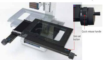
The stage movement can be switched between extremely coarse and fine (FREE and LOCK) by using the quick release handles on the X and Y handles. These handles are useful for freeing the stage when the distance to the measurement position is long or you want to quickly return to a reference position.
